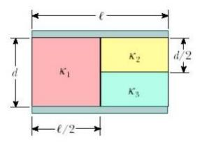
The capacitor can be regarded as being consisted of three capacitors,  $C_1 = \frac{\kappa_1 \varepsilon_0 A/2}{d}$ ,  $C_2 = \frac{\kappa_2 \varepsilon_0 A/2}{d/2}$  and  $C_3 = \frac{\kappa_3 \varepsilon_0 A/2}{d/2}$ , with  $C_2$  and  $C_3$  connected in series, and the combination connected in parallel with  $C_1$ . Thus, the equivalent capacitance is
